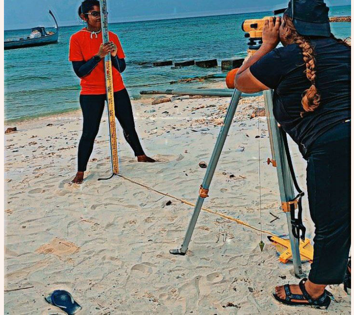
Beach profiling works at the western beach of K. Huraa, using an auto level and a telescopic measuring staff.
