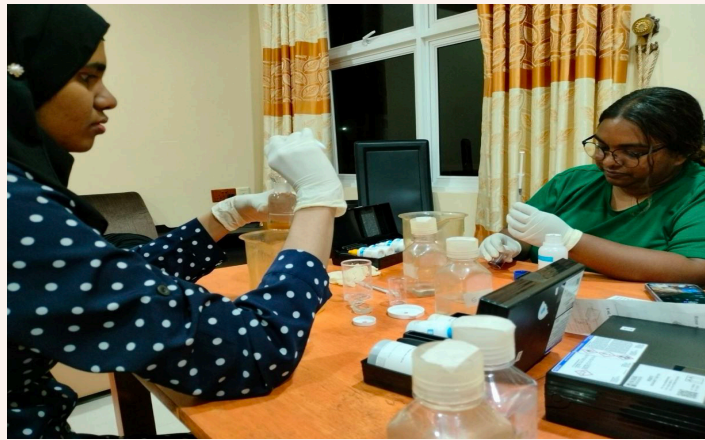
Testing dissolved oxygen content of ground water samples collected using test kits
